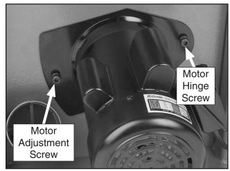
Figure 57. Motor mount screws.
